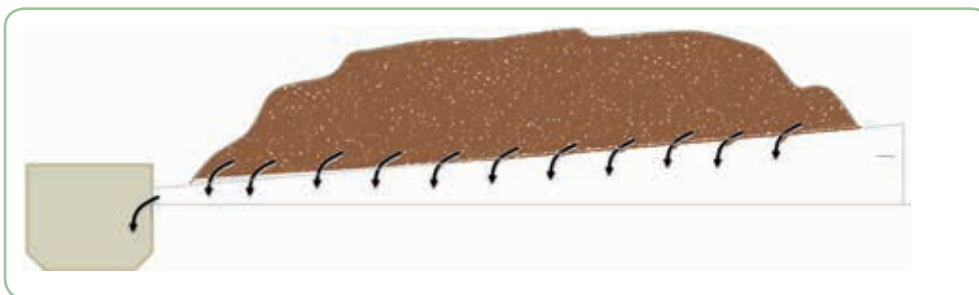
Figure 12 Leaching collection system
